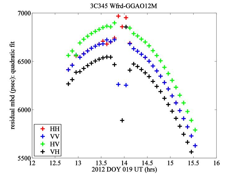
Residual delays to correlator model spanning 2 GHz bandwidth
