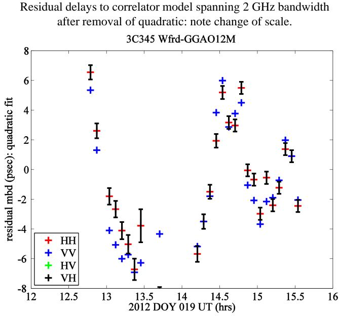
Difference of delays across 2 GHz for vertical and horizontal polarizations. Receiver noises in VV and HH are independent. Note that scale is  $\pm 4$  psec, which is goal for RMS delay variation for VLBI2010. Three picosec = 1 mm.
