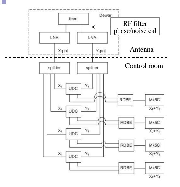
Feed and LNAs cooled to ~20K Both senses of linear polarization used
