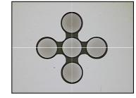
Fiber Pattern at telescope focal plane
