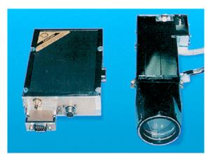
Diode pumped Nd:YAG laser 1064 nm, 170 mJ/pulse, 0.6Hz and 8Hz 10 cm telescope diameter Si APD photodetector 2.4 kg, 6.8W
