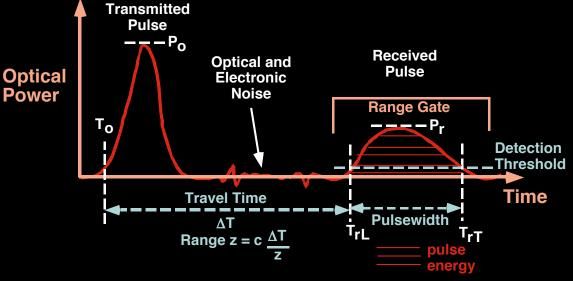
Range -> Elevation Pulsewidth -> Surface roughness Received/Transmitted Pulse Energy ->Surface reflectivity
